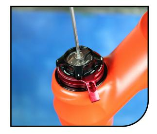
Remove the black high speed compression knob while keeping the silver HBO knob in place.
