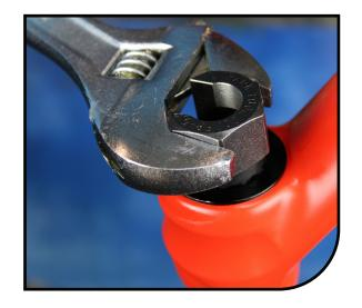
Remove compression damper assembly from the stanchion.
