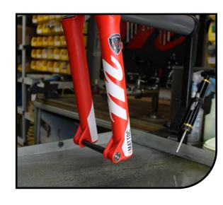
Unscrew air cap and depress Schrader Valve a few times to ensure all air is released.
