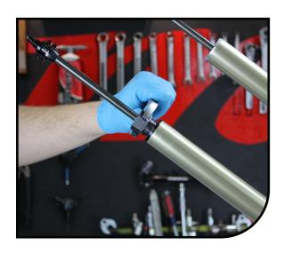
Remove Air Spring Assembly, clean with isopropyl, and re-grease.
