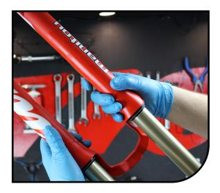
Insert semi-bath into each casting leg. Once the semi-bath is in the legs slide the casting the rest of the way onto the stanchion assembly.
