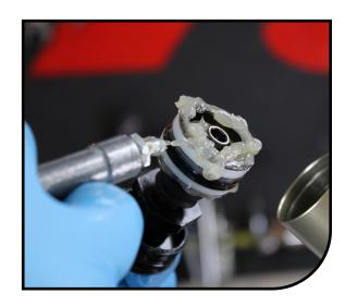
Add Slickoleum $^{\rm TM}$  grease to the stanchion threads before inserting the air spring assembly. Spread grease across entire thread surface.
