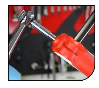
Insert a 8mm Hex wrench into the end of the rebound rod and loosen clockwise until rebound rod disengages from the casting threads.
