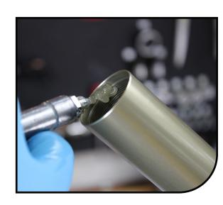
Install air spring assembly into stanchion. Using a 26mm crow's foot and Manitou cassette tool, torque to spec.
