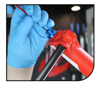
Using the Mattoc 8mm Thin Wall Socket, turn the compression rod **clockwise** until compression rod is disengaged from the casting threads.
