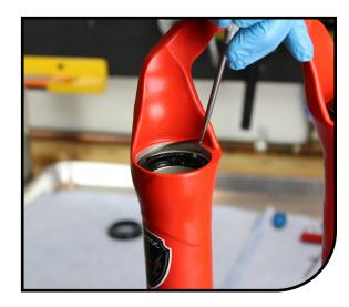
Gently pry the oil seals out of the casting. Place a towel under the tire lever to prevent damage to the casting.
