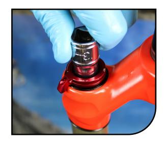
Place high speed and HBO knob assembly onto the red low speed adjustment knob. Tighten down screw with 2mm Hex wrench.
