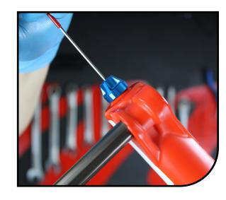
Using the Manitou 8mm Thin Wall Socket, turn the compression rod **counter-clockwise.** Do not overtighten, doing so can damage the end of the rods.
