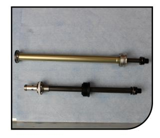
Use a 26mm crow's foot, Manitou cassette tool, and torque wrench to install the rebound damper assembly.
