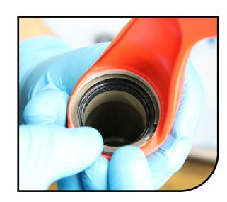
Using the Manitou 34mm Seal Press or large socket press in the dust seals.
