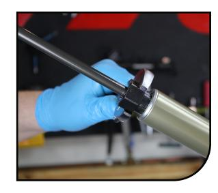
Remove rebound damper assembly from the fork. Once the damper assembly is removed, clean the inside of the stanchion with isopropyl alcohol and a lint free towel. Inspect the inside and outside of the stanchion for scratches and other damage. Inspect rebound damper for damage as well. Replace if necessary.
