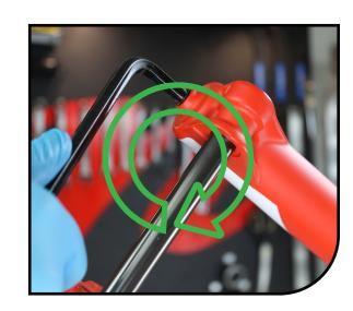
Remove casting from fork. It is recommended this be done over a drain pan as the lower casting contains semibath oil. Allow oil in casting to drain out before continuing to next step.
