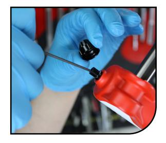
Remove IVA using a 24mm socket.
