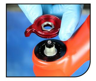
Remove the sliver spacer that was under the red low speed adjustment knob.
