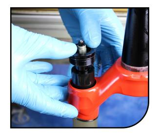
Using a crow's foot, Manitou cassette tool, and torque wrench, tighten down the MC2 at a torque of 60-80 in lb [6.8–9.0 N m].
