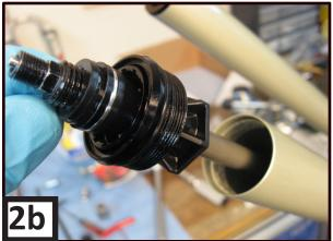
4. Using the Mattoc Cassette Tool and a torque wrench (a socket will fit over the Cassette Tool, shown in picture) tighten the compression rod end cap down to: 60-80 in lbs. [6.8-9.0 Nm]
