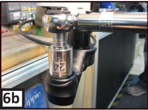
7. Invert fork and attach shock pump to the air valve. Depress the air release button on the pump and pull compression rod out to fully extended position. If your shock pump does not have an air release button use a 3mm Allen wrench to depress valve core and extend compression rod.
