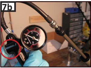
8. Using a shock pump pressurize the air chamber. Put in 20-50 PSI.
