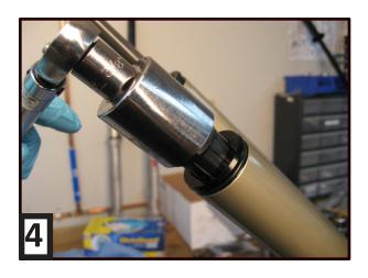
5. Rotate fork to riding position and add a liberal amount of Slickoleum™ grease into the stanchion on top of the compression rod air piston.
