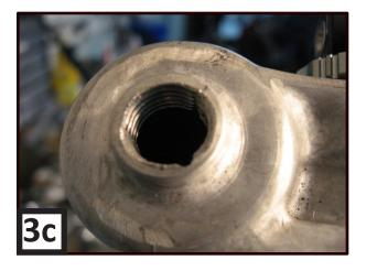
4. Using the Mattoc 8mm Thin Wall Socket, turn the compression rod **clockwise** until compression rod is disengaged from the casting threads.
