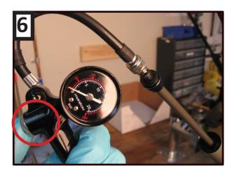
7. With shock pump still attached and pressure release button depressed, compress the compression rod assembly into the upper stanchion of the fork. Compress rod until bottom out bumper is contacting the end cap. If your shock pump does not have a pressure release button use a 3mm Allen wrench to depress the valve core while pushing compression rod into stanchion.
