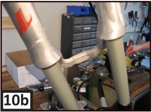
11. Insert Manitou Semi-bath oil into each side of the casting.
