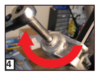
5. Remove casting from the fork. It is recommended that this be done over a drain pan as there is semi-bath oil in the lower legs that will be released when casting is removed.
