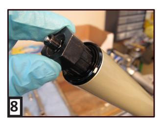
9. Using an adjustable wrench or similar tool, turn the cassette tool counter clockwise to remove compression rod assembly from fork stanchion.
